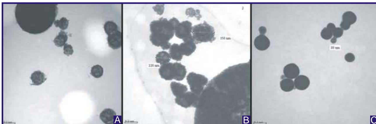
Figure 1 Phytate colloid filtered through 0.1 \mu\text{m} filter (Left panel). The size increased to >200 nm in 2 hours time. The figure in the middle panel shows Phytate colloid filtered through 0.1 \mu\text{m} filter. The size was increased to about 350 nm in 27 hours. The figure on the right panel shows Phytate colloid filtered through 0.22 \mu\text{m} filter. The colloid size was increased to about 220 nm in 2 hrs.
